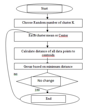
Figure. 1: K-Mean Clustering process
