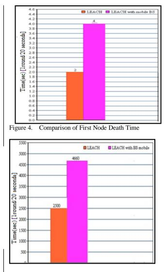
Figure 5. Comparison of Half Nodes Alive Time
