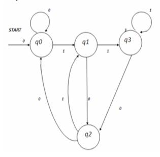
Figure 1 Moore machines which calculates residue mod 4.
