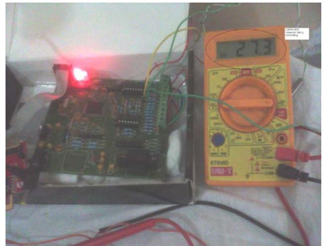
Figure. 5. Current Measurement in Transmitting Mode
