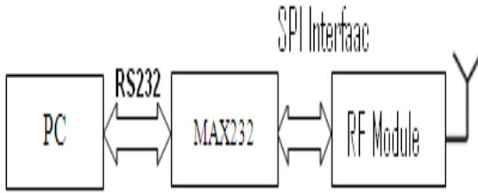
Figure 3 . Block Diagram of Master Mote
