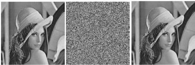
Figure 5. Encryption/Decryption of 'lena' plain image using Tinkerbell map
