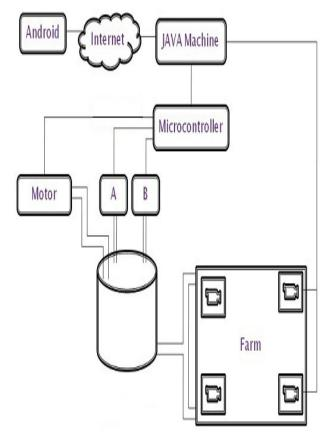
Figure 1: System Architecture
