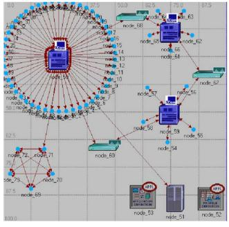
Figure10. Three star topology combination with Mesh
