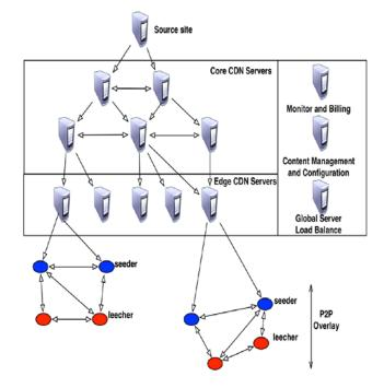
Figure 1.Example model of peer-assisted online storage architecture.
