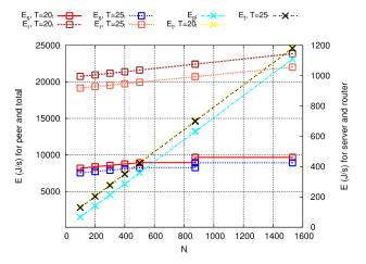
Figure 5. Power consumption for the server, router, peer and total system for peer-assisted CDN with  $N_s^u = 0.75$ . Note that the server and router energy are plotted using the right hand scale, and the peer and total energy are plotted using the left hand scale.
