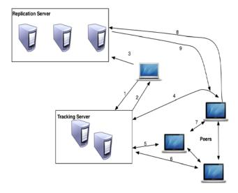
Figure 2.Example model of peer-assisted online storage architecture.
