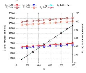
Figure 4. Power consumption for the server, router, peer, and total system for CDN architecture. Note that the server and router energy are plotted using the right hand scale, and the peer and total energy are plotted using the left hand scale.
