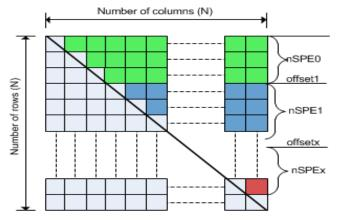
Figure 2. Splitting the matrix of distances to the SPE processors
