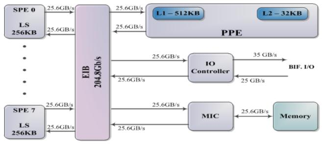
Figure 1. Cell Broadband Engine Architecture[3]
