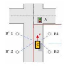
Figure. 2 Pair of transmitter receiver mounted on lane sides to control the traffic
