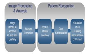
Figure.4. Block diagram for optical character recognition
