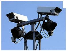
Figure. 6. Camera Used In ANPR Technology
