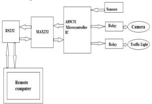
Figure.1. Block diagram of transmission information from lane location to remote computer
