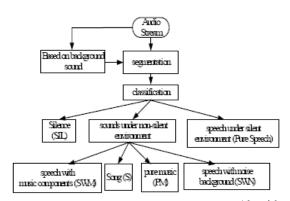
Figure2: The flowchart of segmentation and classification Algorithm
