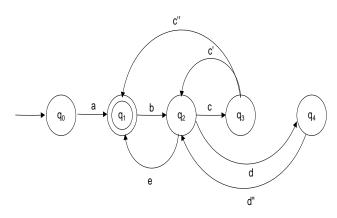
Figure. 4 Finite State machine for Issuing Policy
