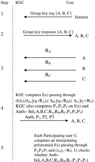
Figure 2 Key Generation and Distribution Process
