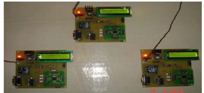
Figure 3 Actual photo of Remote Monitoring System
