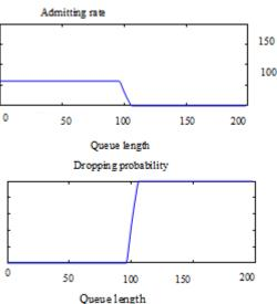
Figure. 6. Optimal admitting instructions rate and dropping probability v.s. processor's queue length, when b = 60 (inst/sec).
