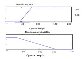
Figure. 4. Optimal admitting instructions rate and dropping probability v.s. queue length, when W=0.1.
