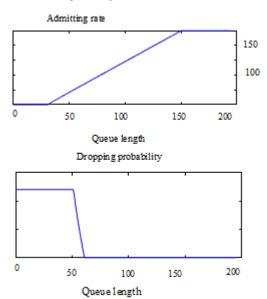
Figure. 5. Optimal admitting instructions rate and dropping probability v.s. processor's queue length, when W = 1.0.
