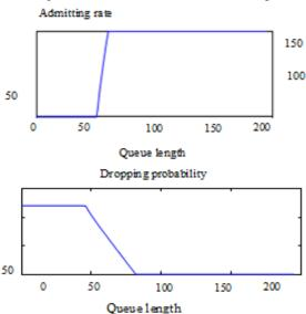
Figure. 3 Optimal admitting rate and dropping probability v.s. queue length, when W=0.01
