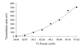
Figure 2. Tx power and their corresponding transmission area
